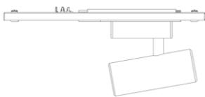
Track Spot light with pre-assembled connector make it easy to joint linear trunking rail electrically and mechanically. Track spot light has three separate switchable circuit—N and L1, N and L2, N and L3. The head of Track Spot light can be rotated horizontally 360°, and adjust vertically 90°.
